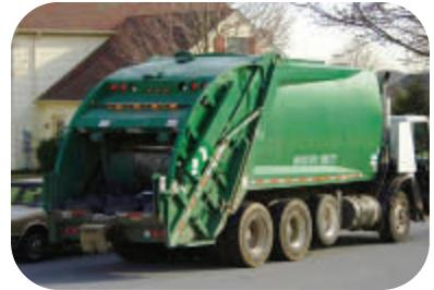
Large vehicles (trucks and some equipment) have extremely limited visibility. A large area behind the vehicle is invisible even with rear view mirrors properly adjusted. This invisible area is called the "cone of invisibility." The larger the vehicle, the larger this cone of invisibility becomes. The driver must become familiar with the cone of invisibility so that precautions can be taken to avoid backing accidents.
