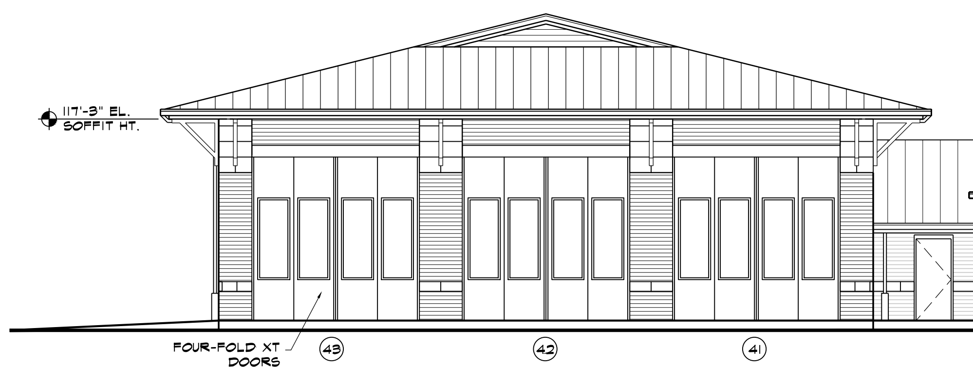
H BID ALTERNATE NO. 2 - BIFOLDING DOORS EAST ELEVATION (FACING EDGEWOOD) SCALE: 1/8" = 1'-0"
