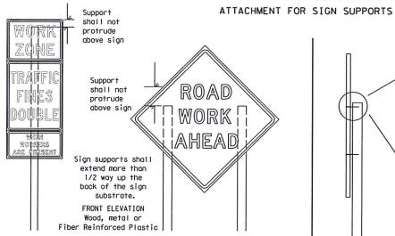
Splicing embedded perforated square metal tubing in order to extend post height will only be allowed when the splice is made using four bolts, two above and two below the spice point. Splice must be located entirely behind the sign substrate, not near the base of the support. Splice insert lengths should be at least 5 times nominal post size, centered on the splice and of at least the same gauge material.
