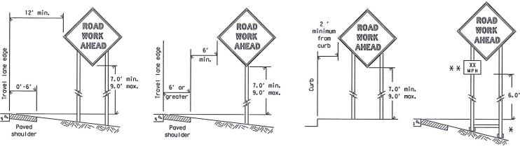
\* When placing skid supports on unlevel ground, the leg post lengths must be adjusted so the sign appears straight and plumb. Objects shall NOT be placed under skids as a means of leveling.
