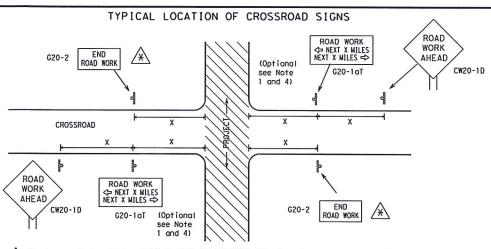
$\nearrow$  May be mounted on back of "ROAD WORK AHEAD" (CW20-1D) sign with approval of Engineer. (See note 2 below)
