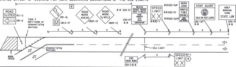
The Contractor shall determine the appropriate distance to be placed on the G20-1 series signs and "BEGIN ROAD WORK NEXT X MILES" (G20-5T) sign for each specific project. This distance shall replace the "X" and shall be rounded to the nearest whole mile with the approval of the Engineer No decimals shall be used.
