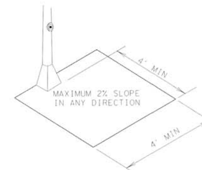
CLEAR GROUND SPACE ADJACENT TO PEDESTRIAN PUSH BUTTON
